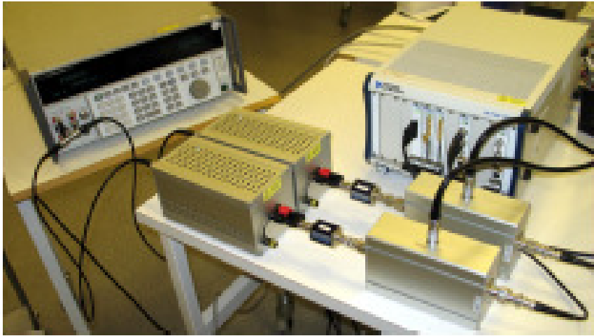
SP phase measuring system for voltage dividers
